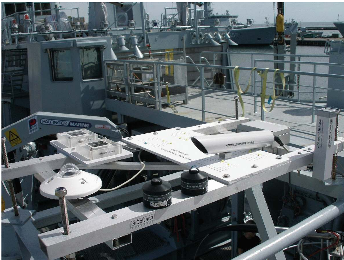
Figure 2: The optics table was an aluminum frame firmly fastened to the aft port side of the vessel near the rail. The sky luminance sensor (at right) points towards the horizon with an elevation angle of about 10 degrees. The two SolData photovoltaic pyranometers are visible at the left rear behind the Kipp-Zonen CM 11.
